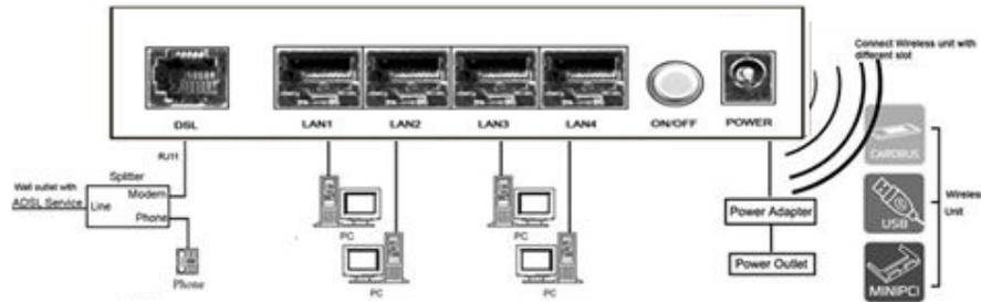
**Notes:** Without the splitter and certain situation, transient noise from telephone can interfere with the operation of the Router, and the Router may introduce noise to the telephone line. To prevent this from occurring, a small external splitter must be connected to each telephone.
