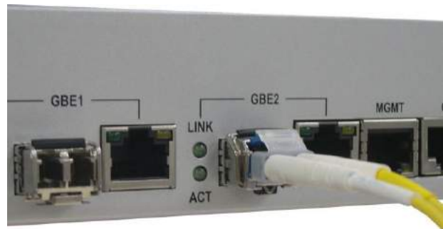
Figure 1-13 Connecting optical fiber to the trunk port
