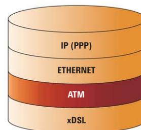
In recent times though, native IP (or IP over PPP) over Ethernet over DSL - or Ethernet in the First Mile implementations are increasingly being adopted by DSL service providers. Without the ATM layer overhead, local loop segments become more efficient and cost-effective.
