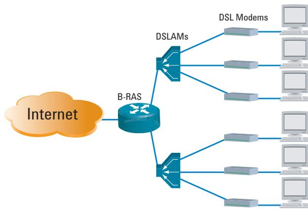
This is an extremely simplistic outline of the DSL access network flow but it carries the message that what really makes DSL happen are the DSL modems and DSLAM and B-RAS devices.
